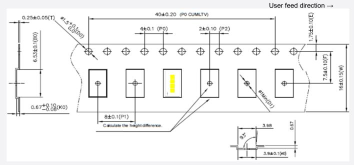
Package placement condition in a reel tape
