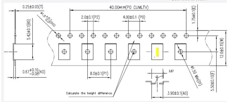
Package placement condition in a reel tape
