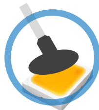
Use vacuum tweezer case (have to keep clean vacuum pad side)
