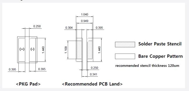
Notes: mm, Tolerance:  $\pm 0.10$  mm, recommended stencil thickness 120  $\mu m$
