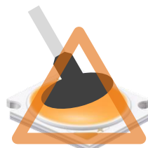
Use vacuum tweezer case (have to keep clean vacuum pad side)
