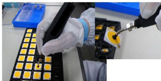
Use vacuum tweezer case (have to keep clean vacuum pad side)
