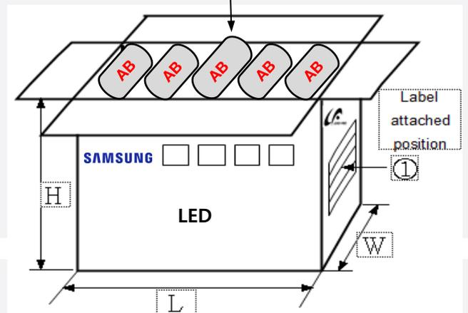
d) Packing Process for kitting (The quantity of PKG on the Reel to be Max 16,000 pcs)
