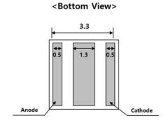
Measurement unit: mmTolerance: ±0.15 mm
