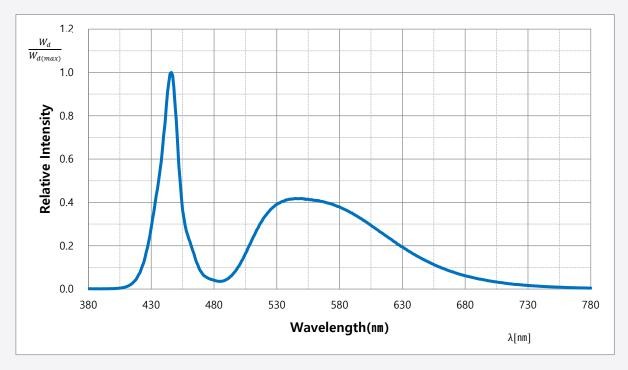
Note: The red content of the light (610~780nm) >5% according to ECE regulation
