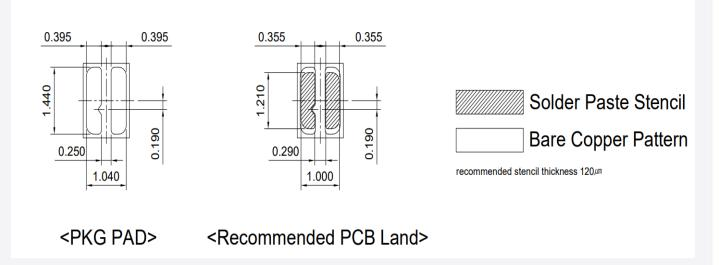
**Notes:** mm, Tolerance:  $\pm 0.10$  mm, recommended stencil thickness 120  $\mu$ m
